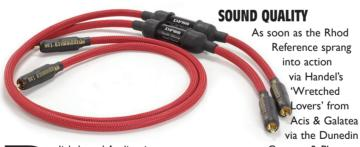
olish-based Audiomica has been around the hi-fi industry for ten years and specialises in cables. Installed to tackle electromagnetic distortion, each cable includes a bulky filter placed halfway along the length. The Rhod Reference features the same DFSS (Double Filtering Signal System) found on the Borax Gold but also includes the company's DSS (Double Screening System) which isolates each conductor to prevent cross-contamination. The cable is also hand-terminate with a gold RCA plug.
